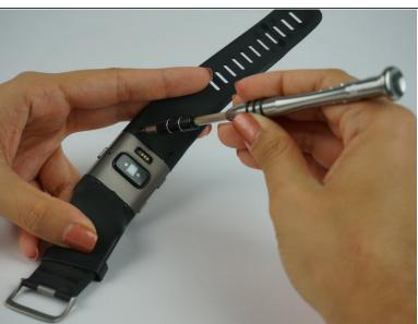
Unscrew all four black 3 mm Phillips screws on the underside of the watch using a T5 screwdriver.
