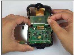
Remove the metal case off of the motherboard.
