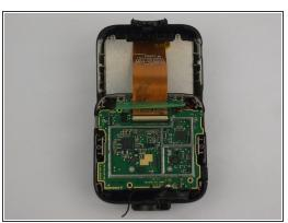
Remove the three 5 mm screws using the Torx T5 screwdriver.
