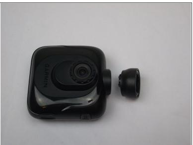
Remove the Dash Cam socket piece.
