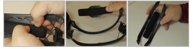
Locate the black wiring and gently pull it out of the plastic headpiece component.
