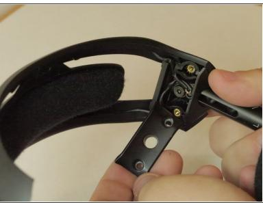
Remove two hex screws on each side to free and remove the base plate. Do each step for both sides.
