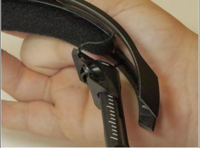
Pull apart earpiece assembly and the connecting headband piece.
