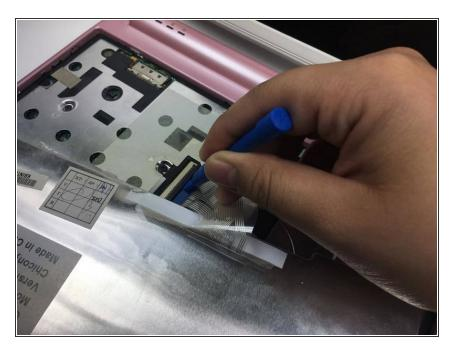
Using the Blue Plastic Opening Tool, pull up on the keyboard connector to completely detach the keyboard from the base of the laptop.
