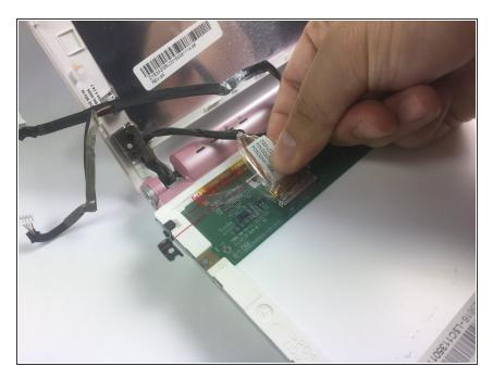
Detach the cord by pulling the cord out of the slot of the green circuit on the bottom of the laptop. Once the cord is detached, the display screen will be unattached and able to be removed.
