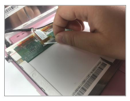
Pull up the transparent piece of tape at the bottom of the display screen that holds the cord in place.
