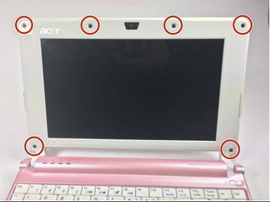
Using a Phillips #1 screwdriver, unscrew the six 5.2mm screws in the places where the rubber coverings were located.
