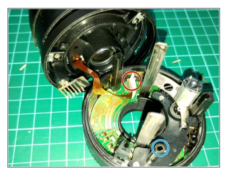
Pull out the connector of the flex cable vertically while supporting the circuit board (I used a plastic spudger to push down the circuit while pulling the white connector). To insert it back, simply push it back into the slot. Note the orientation of the connector (Take lots of pictures)
