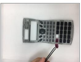
Select which key you need to remove, then using the Angled ESD Tweezers pick up the key, and pull it free from the face plate.
