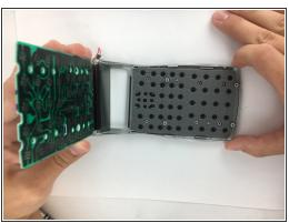
Carefully lift the motherboard, screen, solar panel, and battery terminal combination from the front plate. Start from the motherboard and lift at an angle toward the solar panel.
