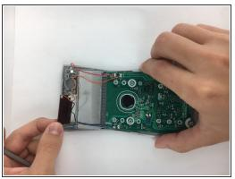
Using the small metal spudger. Carefully pry around the edge of the solar panel until it becomes loose. Then simply pull it from its socket using your hands.
