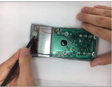
Using the pointed end of the nylon spudger, carefully pry an edge of the battery, and lift the battery from its socket.
