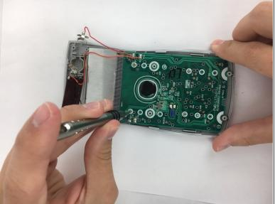
Using a PH0 phillips screwdriver, unscrew the four, 4mm, pan head screws from the motherboard.
