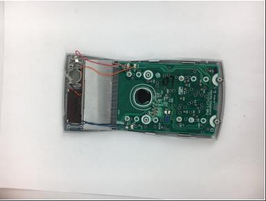
Using the plastic spudger, carefully pry the battery terminals from the front plate. If the plastic spudger is too weak for prying out the terminals, use the small metal spudger. By Carefully bending and/or prying the little teeth on the terminals upwards you can easily remove them.
