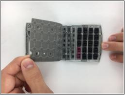
Starting from one corner of the keyboard mat, slowly peel the mat from the front plate and individual keys.
