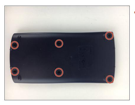
Remove the 6 screws, which are5mm long, using a PH1 screwdriver.
