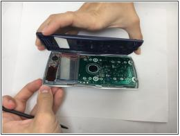
Use plastic spudger to separate backplate from the front-plate. Place the flat end of the spudger in the seam between the front and back, near one end of the calculator. Then slide the spudger towards the calculator's center. The two sides will pop free from each other as you go through it with the spudger.
