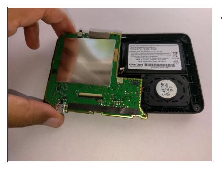
• Tilt and slide the motherboard out of the back cover.
