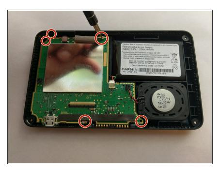
Using a T5 Torx Screwdriver, unscrew the 5 screws holding the motherboard in place.
