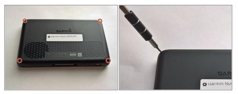
• Using a T5 Torx Screwdriver, begin unscrewing the four 11.0 mm screws from the back panel.
