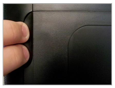
• Insert 2 finger in the dent on the right side of the printer and pull towards the front of the printer.
