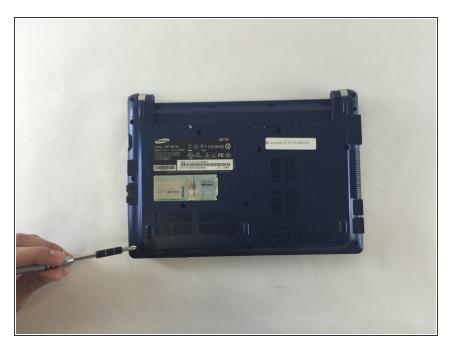
Locate the 14, 3.93 mm, screws that need to be removed on the base of the computer.
