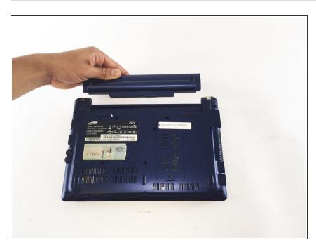
Pull the battery up from the device.
