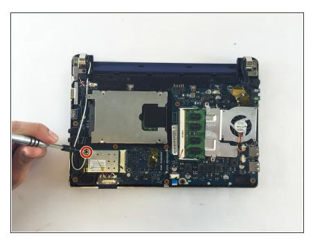
Using a 3.93mm Phillips screwdriver remove the screw attaching the WLAN card.
