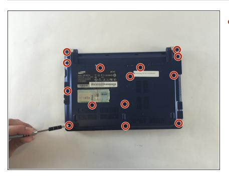
Remove all 14 of the 3.93 mm screws using a PH1 screw bit.
