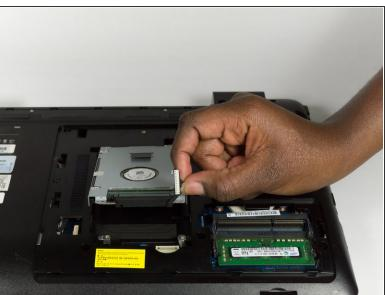
Pull the cord that connects the Hard Drive to the Motherboard to disconnect it.
