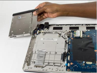
Remove the Optical Drive by sliding it away from the laptop.
