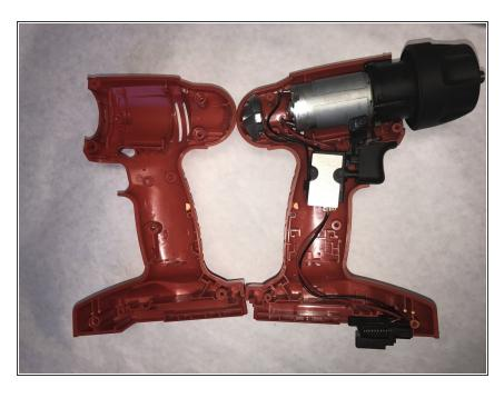
Separate the outer drill case to expose the components and switch. To reassemble your device, follow these instructions in reverse order.
