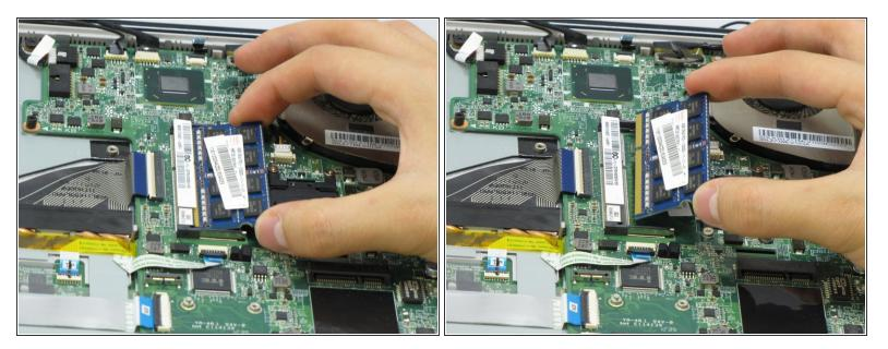
• Continue to pry open the clips, and slip the RAM from its housing.
