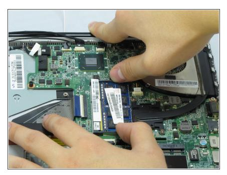
• Pry the RAM's two holding clips in an outward motion.
