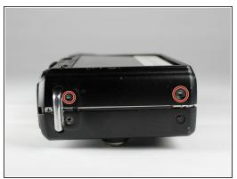
Using a Phillips #00 screwdriver, remove six 2.69mm, silver screws located on the two short sides
