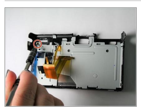
Using a Phillips #00 screwdriver, remove the 3.5 mm silver screw from the upper left hand corner of the back cover.
