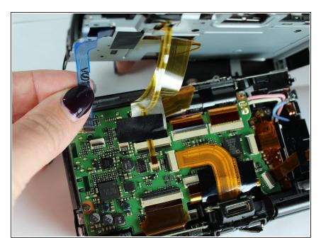
Gently push the blue and yellow ribbons out of the unlocked ZIF connectors using your fingers.
