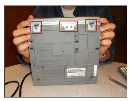
Unclip the three latches on the bottom of the device.
