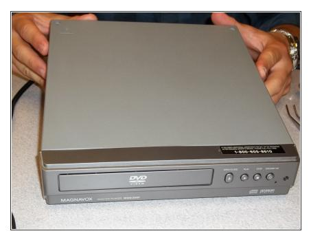
Remove the plastic cover by lifting up the back and pulling it away from the faceplate.
