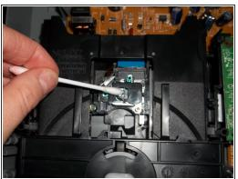
• Locate the optic lens in the middle of the disc drive. Dip a cotton swab in rubbing alcohol and use it to lightly wipe the lens. After the lens is clear of dust and debris, wait a few minutes to let it air dry.
