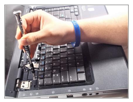
Unscrew the four 2x2 mm screws with a #00 Phillips screwdriver.
