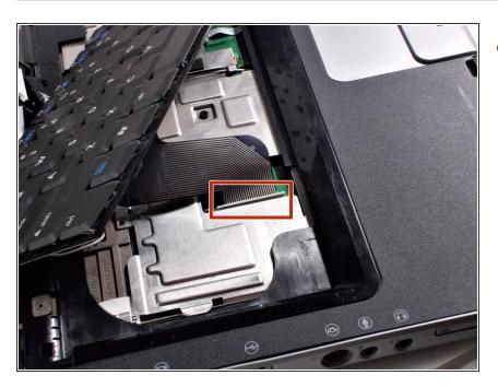
Locate where the ribbon strip is connected to the motherboard.
