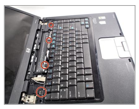
Locate the four 2x2 mm screws that hold the keyboard in place.
