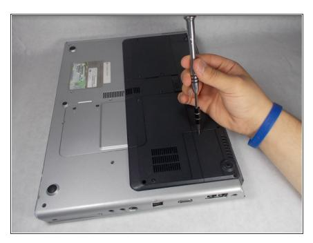
Remove the one 2x5 mm Torx screw securing the thermal cover with a #6 Torx screwdriver.
