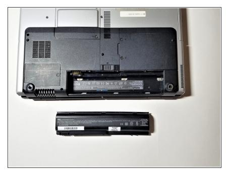
Lift the front edge of the battery up and remove it from the compartment.
