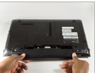
Pull the battery out of the laptop towards yourself to safely remove the battery.
