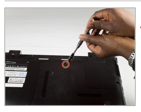
Unscrew the 3.5mm screws using a Phillips J0 Screwdriver by rotating the screwdriver in the counter clockwise direction.
