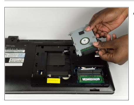
Remove the Hard Drive by lifting it towards you.
