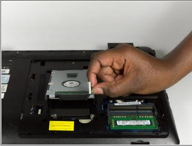
Pull the cord that connects the Hard Drive to the Motherboard to disconnect it.
