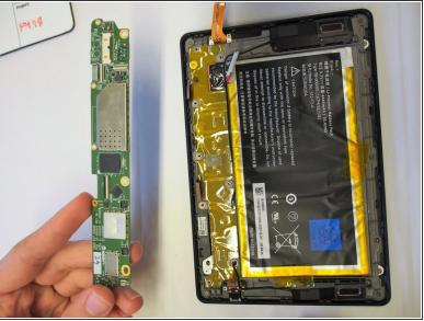
Using the nylon spudger, gently pull up on the motherboard and pull it out of the tablet. The mother board should now be disconnected completely.
