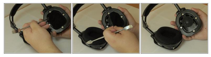
Remove the dust cover located on the speaker. Use the corner of the spudger to peel underneath
