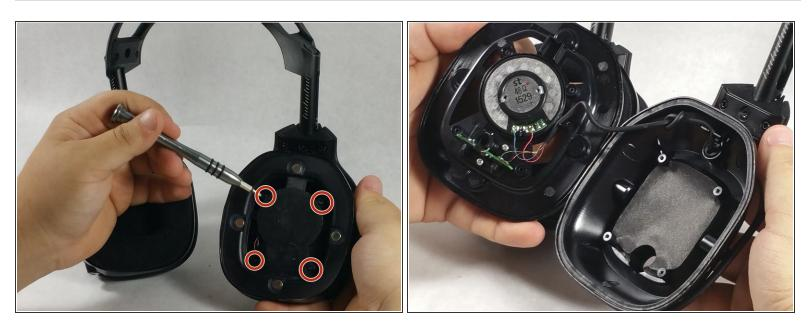
Take off the front cover by removing the four screws located in a square formation on the surface of the device. Use the J00 Philips driver listed in the device page.
