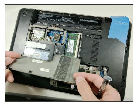
Insert the new RAM inside the same slot the older one was taken out of and put the cover back in place.
