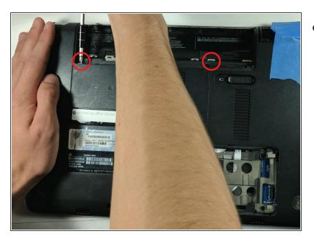
Remove 2 screws securing the cover (as shown in pic)
