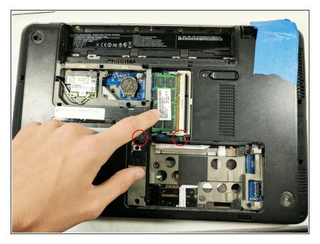
Locate and remove RAM carefully without breaking anything.
