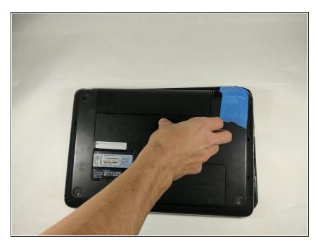
Locate the and remove the battery from device.
