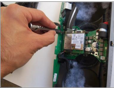
Remove one 7 mm Torx security screw from the top left corner and two 5 mm Torx security screws from the bottom left and top right corners of the circuit board.
