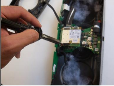
Solder the two wires connecting the circuit board to the motherboard.
