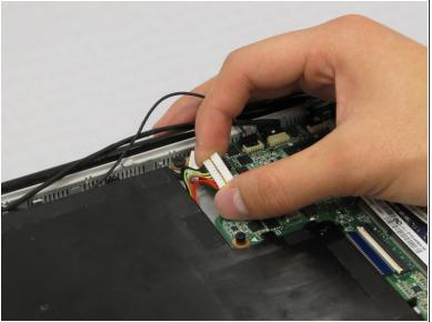
Unplug the Battery from the circuit board by carefully prying the connector from its housing.
