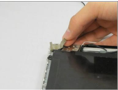
• Lift the strip tape away from the battery, being careful not to completely remove it.
