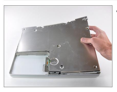
Lift the bottom shield off.
