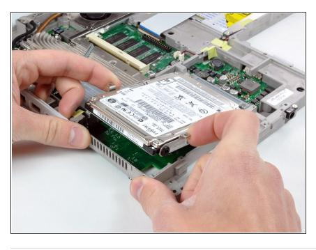
Lift the free end of the hard drive up, enough for the brackets to clear the metal frame. Pull the hard drive out of its connector.
