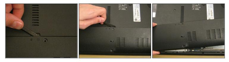
• Use a spudger to release the panel from the plastic retaining clips keeping it in place.
