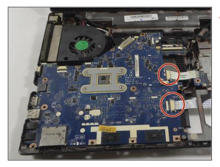
Remove the two remaining ribbon cables as described in Step 11.
