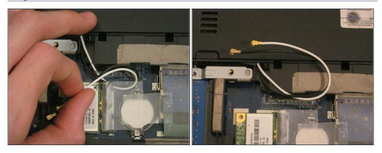
② You may find it useful to pull the antenna cables out from under the plastic retaining clip so you can move them out of the way while you work.
