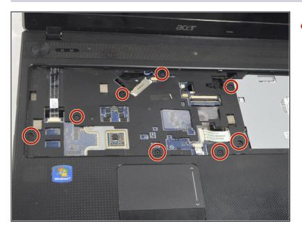
Remove the 8 Phillips #0 screws from under the keyboard.
