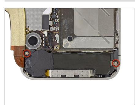
Remove the two 2.4 mm Phillips screws securing the speaker enclosure assembly to the outer case.
