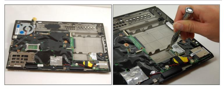
• Remove a total of twenty-three 4.1mm screws from around the black plastic in the board.
