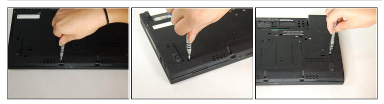
• Remove five 5.7mm screws from the bottom.
