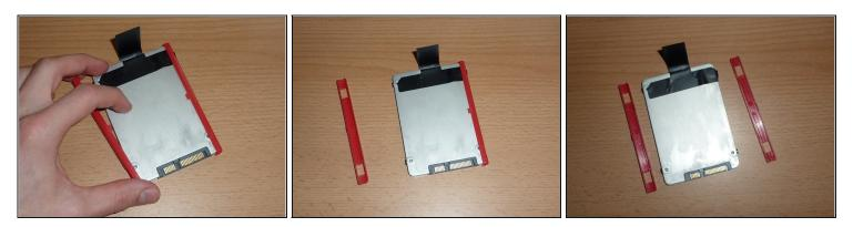
• Remove the plastic rails from the old SSD/hard drive and place them on the new SSD/hard drive.
