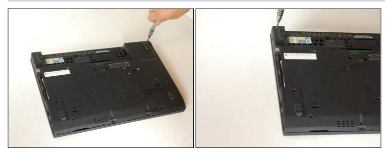
• Unscrew two 5.7mm screws from the top of the bottom of the laptop.
