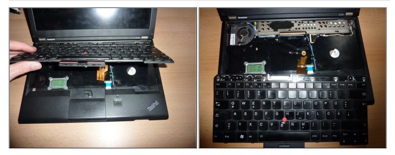
• Carefully lift the keyboard so that you can access its connector.
