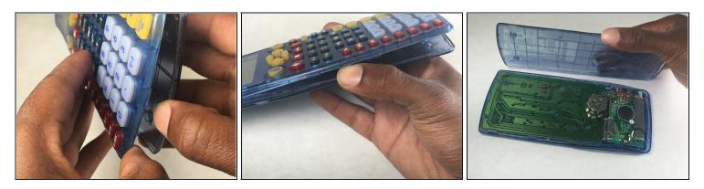
• Separate the two panels to reveal the calculator's green circuit board.
