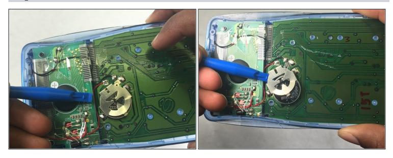
• Using the iFixit opening tool, slide underneath the battery cover until the battery comes out.
