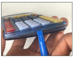
With an iFixit opening tool, pry apart a total of 3 notches on the top and bottom of the calculator.
