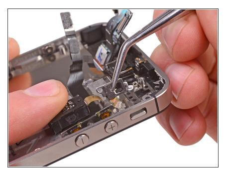
Use a pair of tweezers to gently pull the silent switch bracket away from the outer case.
