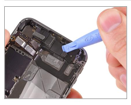
Use the edge of a plastic opening tool to disconnect the Wi-Fi antenna from the logic board.
