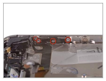
Remove the four 1.5 mm Phillips screws securing the volume button and silent switch brackets to the outer case.
