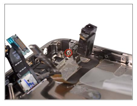
Remove the 1.6 mm Phillips screw securing the mute switch bracket to the outer case.
