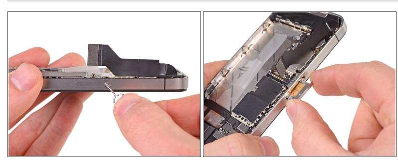
Use a SIM eject tool or a paperclip to eject the SIM and its tray.
