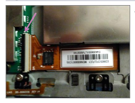
Now the back side is open, disconnect the screen cable from the motherboard as is done in <u>this video</u> from 3:14 until 3:21. Again do not follow the next steps from the video as we don't need them to replace the screen.
