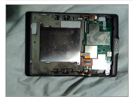
• pull the black tab of the battery connector up and then pull out the cable carefully
