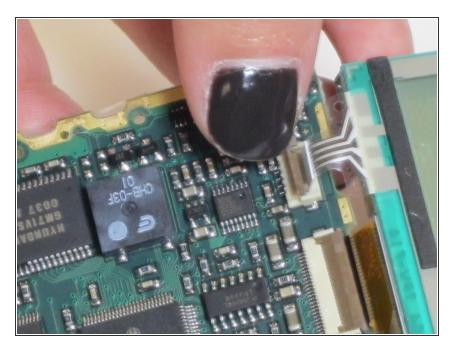
Unplug the three connectors located on the right side of the circuit board with great caution and care. Do not pull by the cable, and be sure to pull the connector itself gently.
