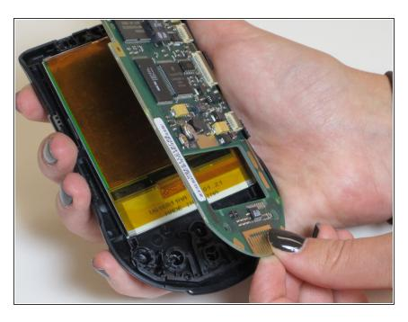
Carefully lift up the circuit board, which will also lift up the screen. Do so carefully to prevent breaking the connectors.
