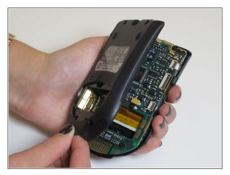
Remove rear cover by gently lifting it up from the bottom.
