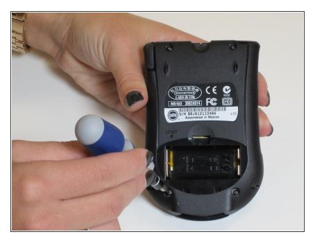
Put the back cover on the device and screw the four screws, screwing in a clockwise direction. Take caution not to over-tighten the screws.
