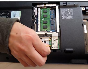
Disconnect the black and white wires on the small circuit board by gently pulling them out of their sockets.
