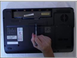
Remove the fifteen screws from the back of the laptop with a Phillips #00 Screwdriver.
