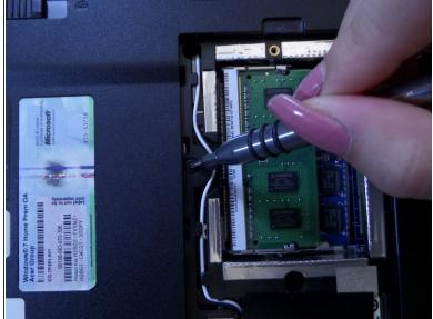
• Remove the two screws on the left and bottom of the circuit board with a #00 Phillips Screwdriver.
