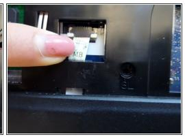
Disconnect the two blue and white ribbons by applying pressure downward and pushing them out
