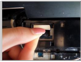
Disconnect the screen connector in the upper left of the laptop.
