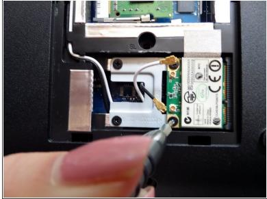
• Remove the four screws from the metal piece beneath the circuit with a Phillips #000 Screwdriver.
