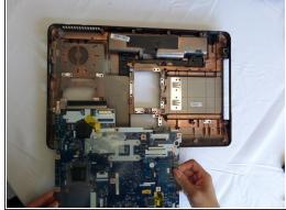
Lift the circuit board out of the back panel and turn it over so the fan is facing up.
