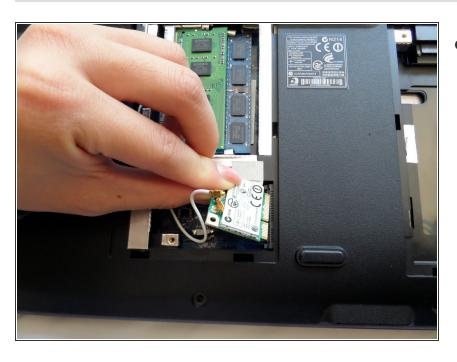
The small circuit board will pop up easily. Carefully remove it
