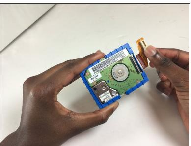
Lift white flap on top of hard drive to disconnect hard drive connector.
