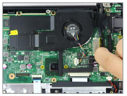
Disconnect the fan's power cable by pulling upward on the pin connector with a pair of tweezers.
