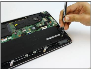
• Use a Phillips 0 screwdriver to remove the eight 5mm Phillips screws holding the battery in place.
