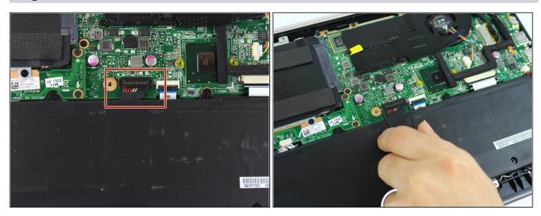
• Remove the ribbon cable with a pair of tweezers.
