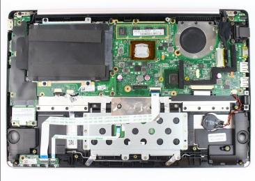
• Grab the sides of the fan assembly and remove it by lifting upwards.
