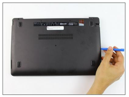
Use a plastic opening tool to pry the back panel off.
