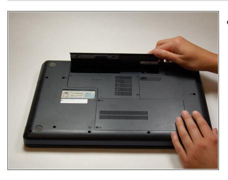
Remove the battery, carefully, from the compartment.
