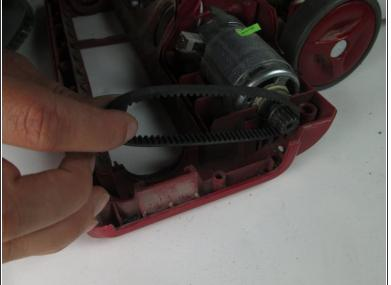
Remove the roller belt from around the roller brush and the motor gear.
