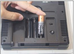
Remove the 3 x AA alkaline batteries from each battery slot.
