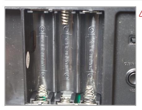
Before replacing the batteries pay attention to the position of the + and - poles on the battery compartment pad.
