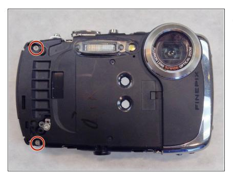
• Using a Phillips #00 screwdriver, remove the two 3.0 mm screws.
