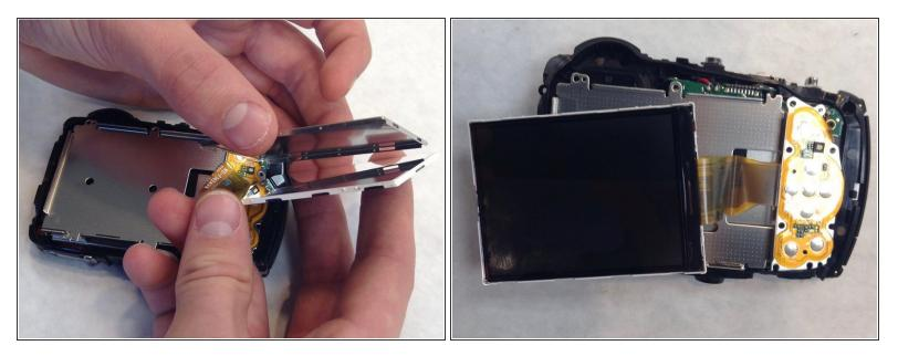
Take the spudger and wedge it very carefully between the LCD screen and the very thin and fragile frame.
