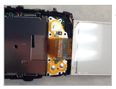
Detach the LCD screen from the motherboard by detaching the orange ribbon.
