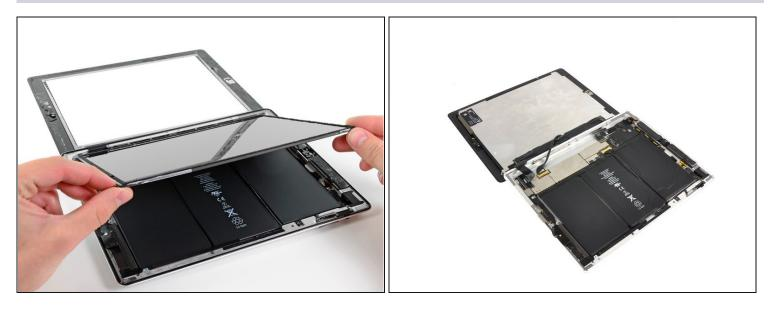
• The front panel ribbon cables are connected beneath the LCD. To access them, you'll need to temporarily flip the LCD over and out of the way.
