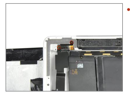
• Remove the two 2.9 mm Phillips screws securing the headphone jack to the rear panel.
