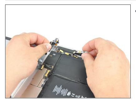
• Carefully peel the front camera cable off the bottom ribbon cable attached to the headphone jack.
