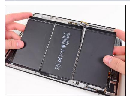
• Carefully lift the battery out of the rear panel and remove it from the iPad 2.
