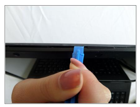
Pop the bezel loose along the edges with a plastic opening tool.
