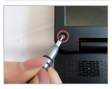
Extract the hidden screws from each of the bezel's four corners, using a #00 Phillips screwdriver.
