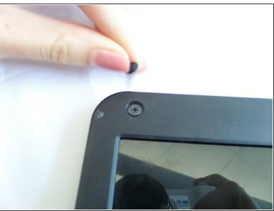
Remove rubber bumpers from each four corners to expose the hidden screws that hold the screen bezel in place.
