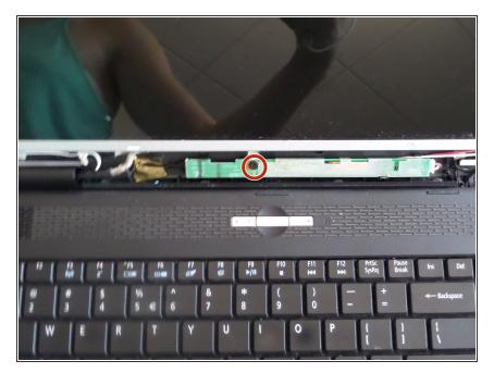
Unscrew the middle screw on the green strip under the screen.
