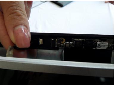
Disconnect wires from the webcam located above the screen.
