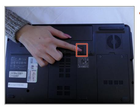
Slide the right latch down to unlock the battery.
