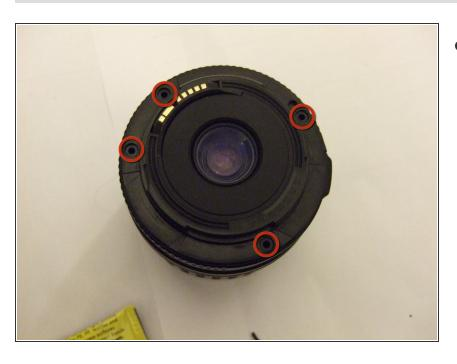
Next, remove the four screws holding the rear cover of the lens on
