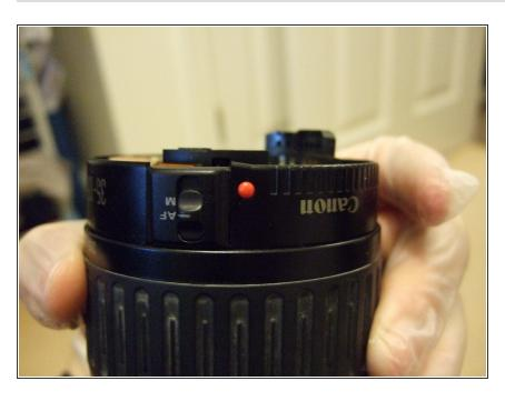
Gently lift and remove the plastic barrel next to the focus switch. My one was already cracked.
