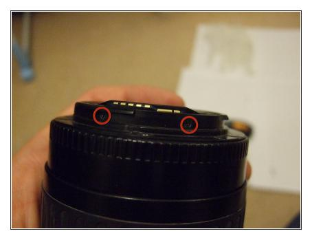
First, remove the two screws in the barrel of the lens with a philips 0 screwdriver
