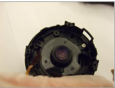
Remove the screws holding the rear element and aperture in place.
