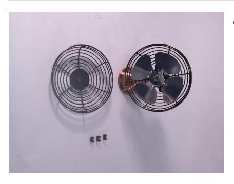
The Guard of the fan is detached from its base due to the effectiveness of a screwdriver.
