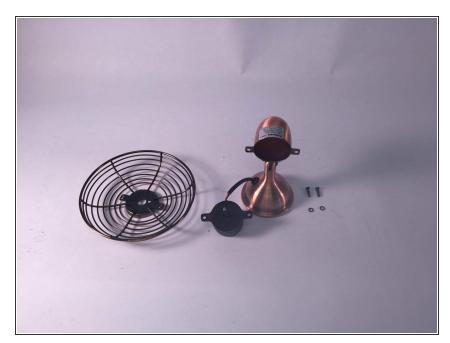
The image to the left of the screen displays the guard of the fan conspicuously detached from the fans base. Various screws are spread across the canvas due to their removal.
