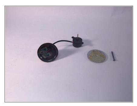
The casing which covered the interior of the motor has now been removed through the use of a screw to gain access to its interior.
