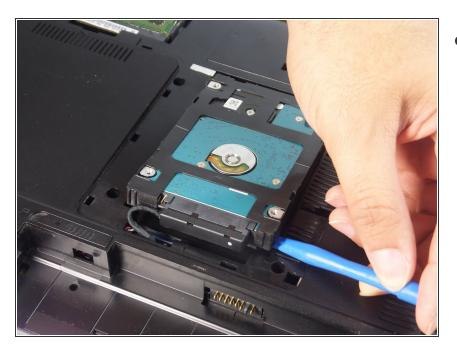
Carefully lift the HDD up using plastic opening tool.
