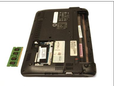
Once the RAM card is propped up, carefully pull it out of its port.
