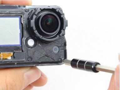
Remove the six T3 Torx screws.
