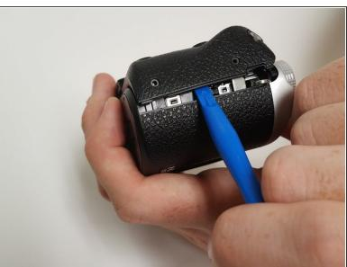
Use the plastic opening tool in a downward motion around each side of the camera to pry the casing open.
