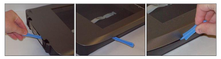
• Push the plastic opening tools into the crack between the top and the bottom of the chassis.
