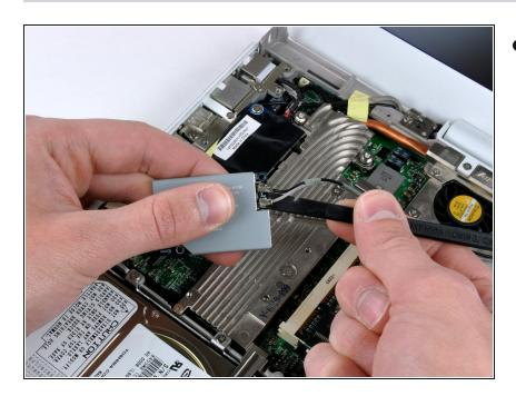
Hold the AirPort/Bluetooth board in one hand and use a spudger to disconnect the two antenna cables.
