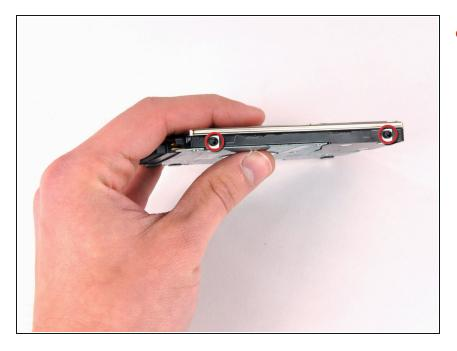
Remove the two black T8 Torx screws from either side of the hard drive (four screws total).
