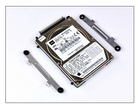
• Remove the hard drive brackets from the left and right sides of the hard drive.
