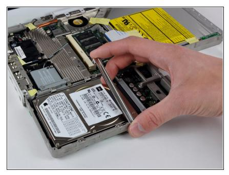
• Remove the metal hard drive retaining bracket from the computer.
