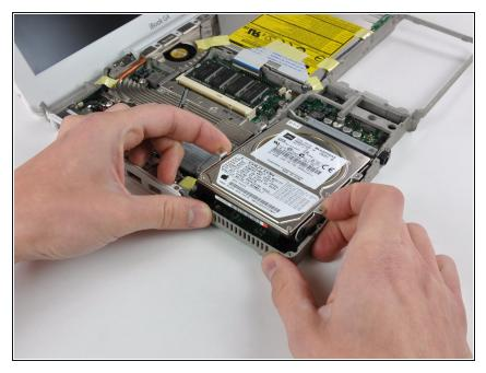
• Slightly lift the hard drive from the free end and pull the hard drive straight away from the connector.
